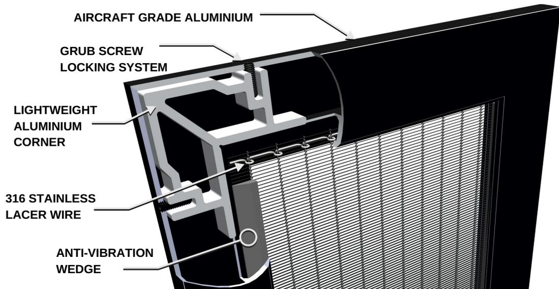
A result of decades of extensive international research and development, MicroLouvre is a high-performance, woven metal fabric, with its weft constructed of bronze louvres. Window covering screens are constructed by tensioning the fabric in aluminium framing and incorporate an anti-vibration wedge to enhance the screen's integrity at wind speeds in excess of 100mph/160kph.
